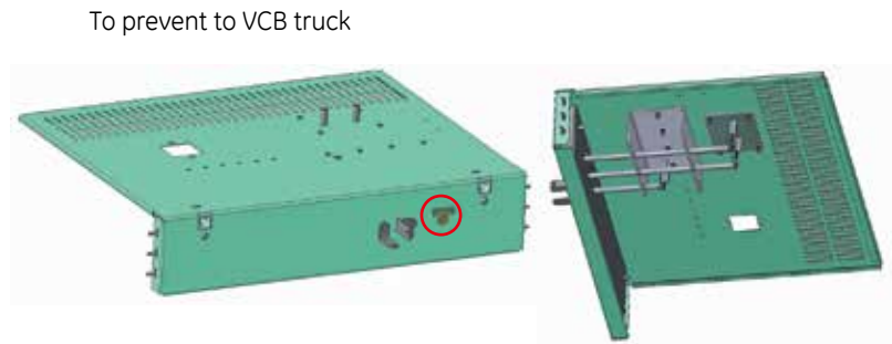
Figure 3.17: VCB trolley Rack-in/out key lock
