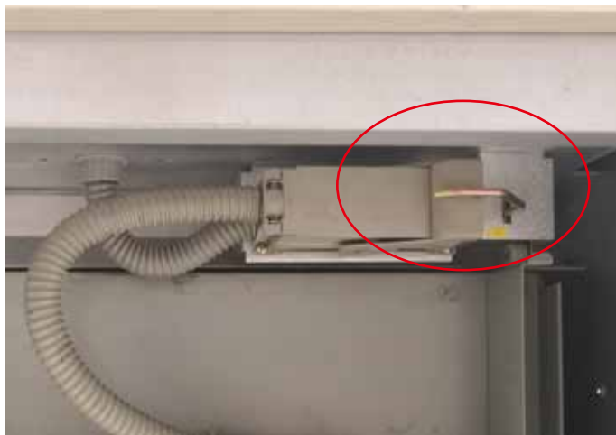
Figure 6.18: Secondary plug latch
