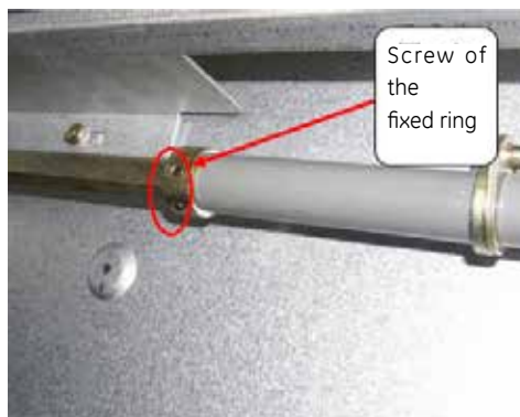
Figure 7.4: Screw of the fixed ring on drive rod
