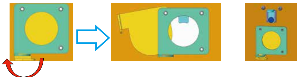
Figure 3.19: Padlock for Circuit breaker racking-in/out operation
